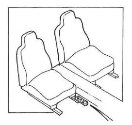
Installation of 7110-1229 Chair Rail Mount to the vehicle chair rail provides an M20 threaded mounting point for Zirkona products.
