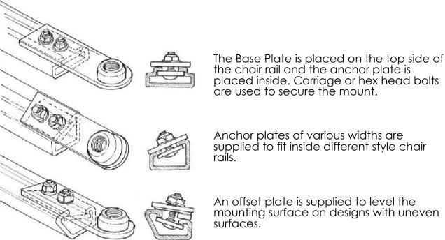
An offset plate is supplied to level the mounting surface on designs with uneven
