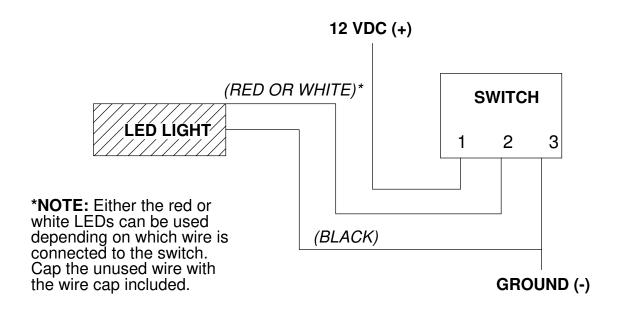
Workstation Light Wiring Diagram
