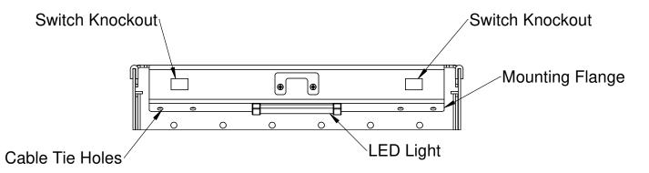
FIG 2 - Workstation Light Mounting
