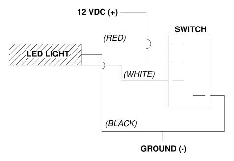
Console Box Light Wiring Diagram
