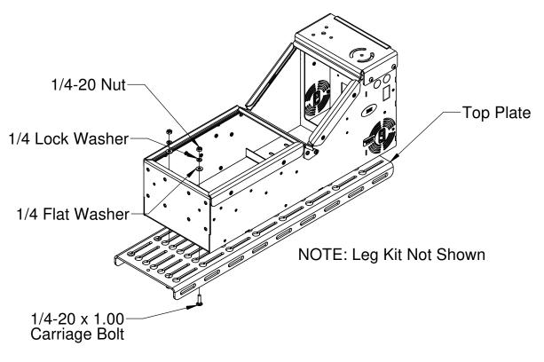
FIG 1 - Console Installation on Top Plate
