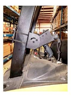
—cap nuts to adjust width
