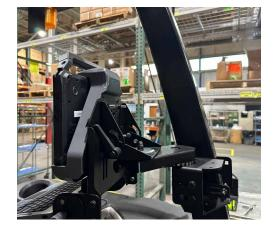
OVERHEAD GUARD LEG MOUNTS **OVERHEAD GUARD LEG MOUNTS**
