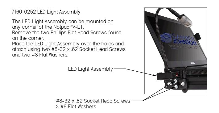
The LED is powered using the red and black wires on the light base. The LED Assembly is designed to operate on 12 VDC.
