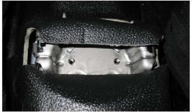
Fig 1 - Rear Mounting Bracket, Carpet Cut to Reveal Threaded Inserts
