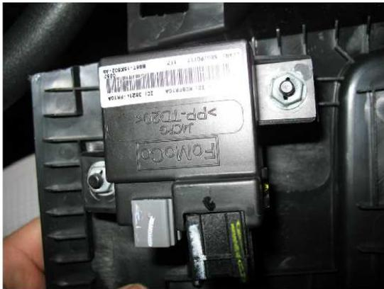
Fig. 3 - OEM Module located on backside of trim Panel
