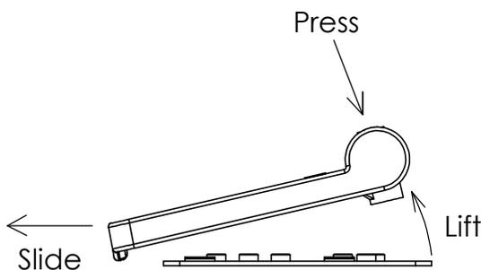
To remove the top quick release plate - press and hold the latch button while lifting slightly and sliding in the shown direction.
