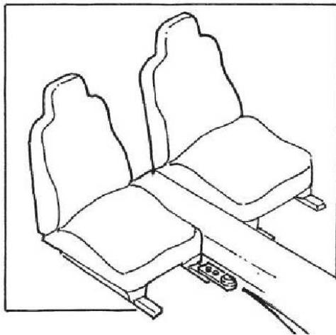
Installation of 7110-1229 Chair Rail Mount to the vehicle chair rail provides an M20 threaded mounting point for Zirkona products.
