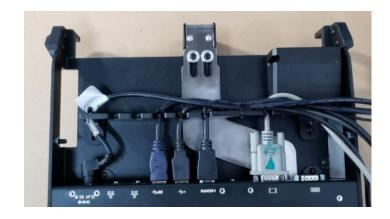
Connect all cables securely to dock ports, and use tie straps to secure cables to the "Cable Management Bar" as shown.
