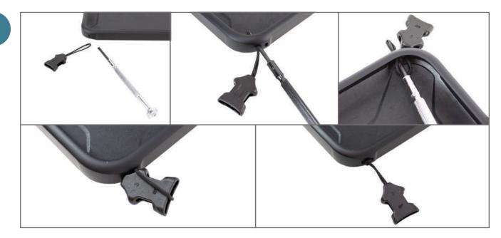
Next, feed the cord of the quick connect clip (3) into the cord slots built into the outer case. **This will require the assistance of a small screwdriver (not included).** Feed the cord inward and then outward (as shown above). With the cord through the slots, loop the cord back around the plastic buckle on the quick connect clip. Pull on the buckle to tighten the quick connect cord to the device.
