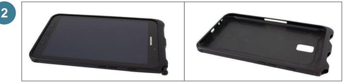
Before installation, please remove the Tab Active2 and stylus from the outer case and set them safely to the side. The mobility bundle will be installed to the outer case.
