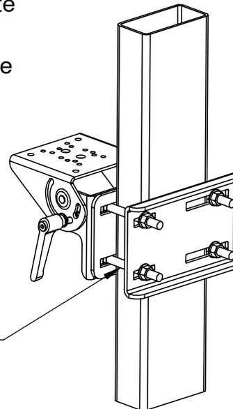
Position the 3/8 carriage bolts as close to the overhead guard leg as possible to prevent bowing of the components
