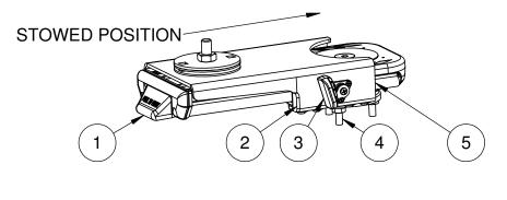
**1 - PIVOT LEVER** 2 - THUMB REST 4 - MOUNTING STUDS
