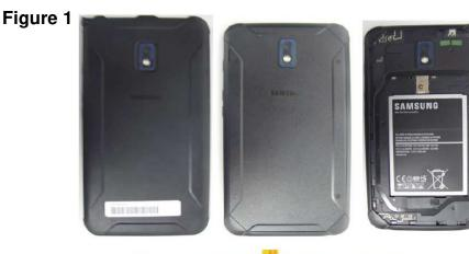
1. Remove the Samsung Tab Active 2 bumper case and back cover. (Figure #1)
