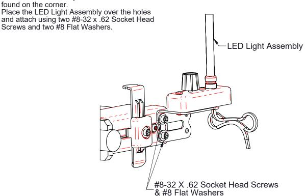
The LED is powered using the red and brown wires on the light base. The LED Assembly is designed to operate on 12 VDC.
