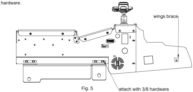
6. with the console in place, the cover wings can be installed in the place attach to console with provided #10 hardware and support brace
