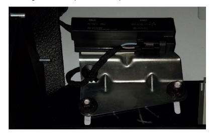
8. Front of the console is installed, align middle of the console with center stud, install the provided spacer under center leg and tighten with OEM nut (fig. 2) \* for 2021+ MY, only need to install 1 spacer
