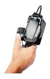
To remove the scanner, push the thumb latch to the left and pull outward on the scanner handle.
