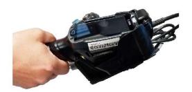
Place the top end of the scanner into the dock at approx. a 45 deg. angle Push upward until it hits the top inside edge where the pins are located.
