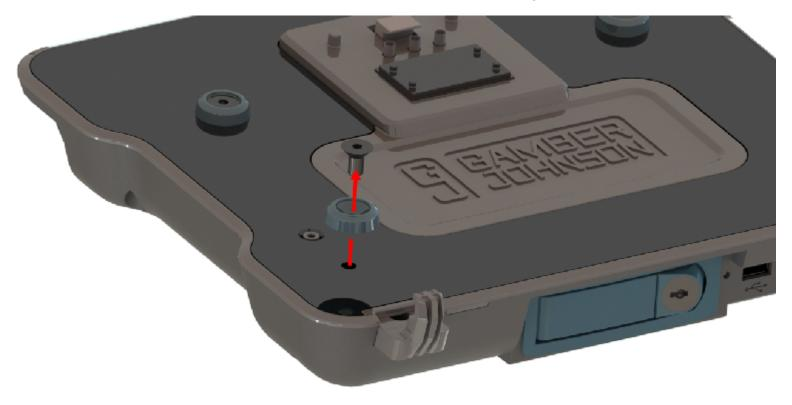
3. Take each blue bumper and insert the bumper in both of the Retrofit Hooks provided in the kit.
