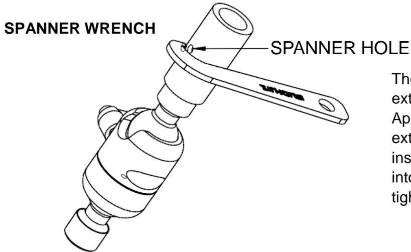
The spanner wrench is used to tighten extension tubes onto the joiner bodies. Apply epoxy thread locker EA 9460 on external and internal M20 threads, then insert the hook end of the spanner wrench into the hole of the extension tube to tighten the joint.
