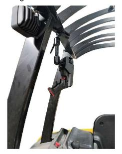
different view showing mount hanging from the overehead guard vs the previous photos mounted off the overhead guard leg
