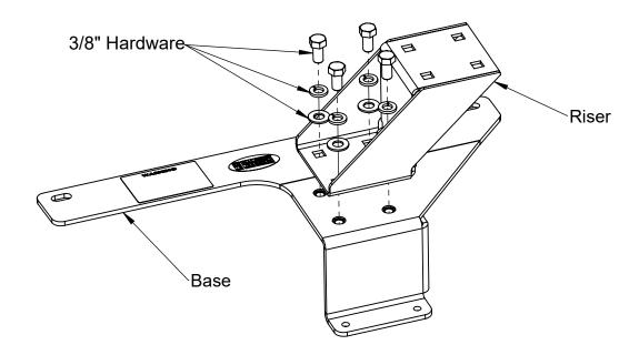
These instructions cover the installation of Gamber-Johnson vehicle base for 2017+ Chevrolet Bolt.
