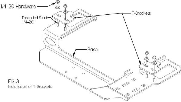
7. With the 1/4-20 hardware fastened, the installation of the base is complete. If installing p/n 7160-0055, add the off-set mounting step (p/n: 7110-0553) to the base as shown in FIG.4 You can then add the desired mounting system (lower pole, upper pole, motion device and computer solution) as needed.
