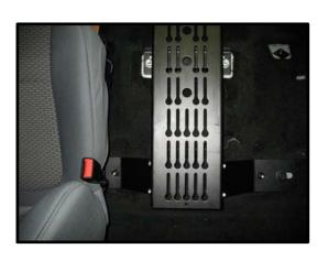
7. Install Workstation and other equipment to the Top Plate as required. Complete the install by reinstalling the passenger seat.
