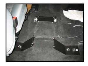
6. Install the Top Plate using (6) .38-16 bolts and washers supplied in hardware bag. Adjust Back Leas so Top Plate is aligned with center of vehicle.
