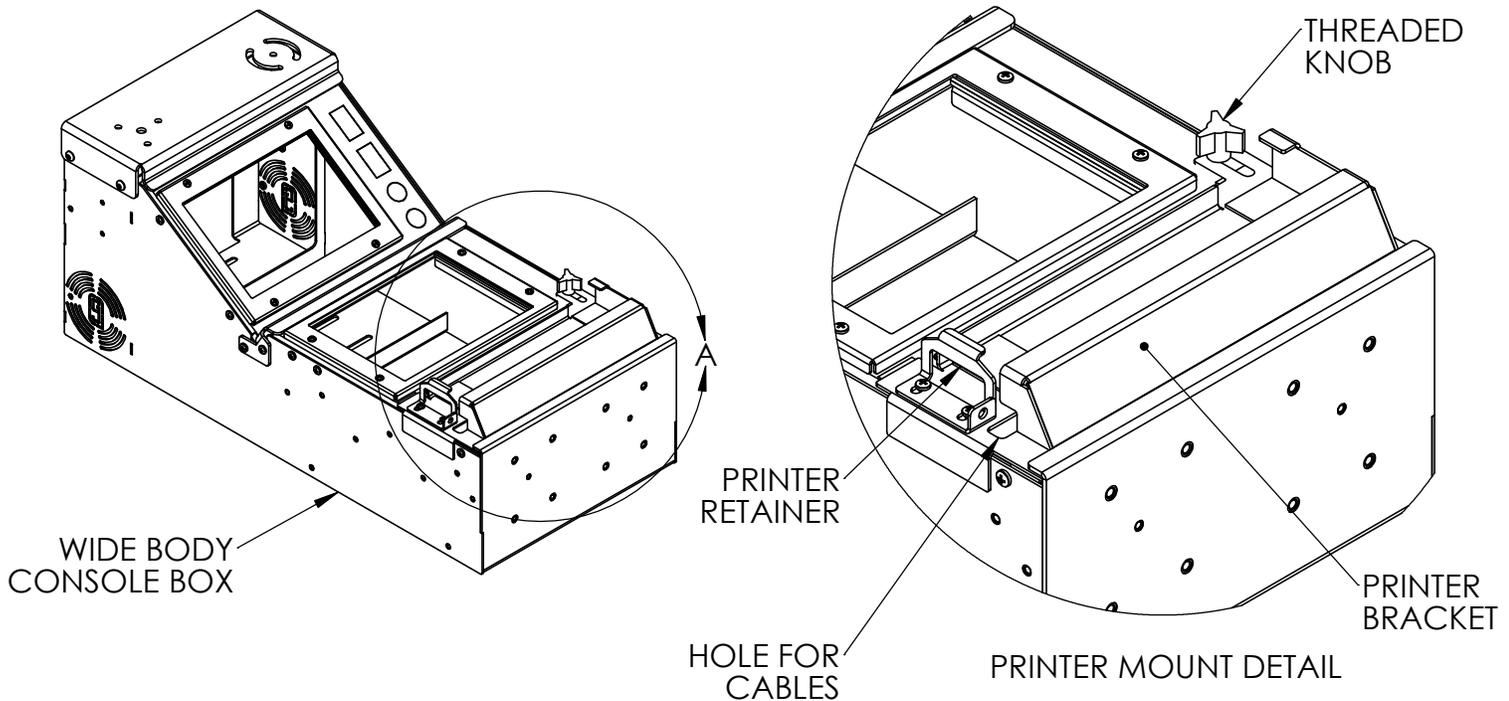
The wide body console printer mount is designed to mount a Brother Pocket Jet series printer and paper within the console box. The printer is mounted near the back of the console box and is removable to access the paper roll for refilling. These installation instructions will cover the general functions of the printer mount as well as how to install the printer mount upgrade into an existing wide body console box.
