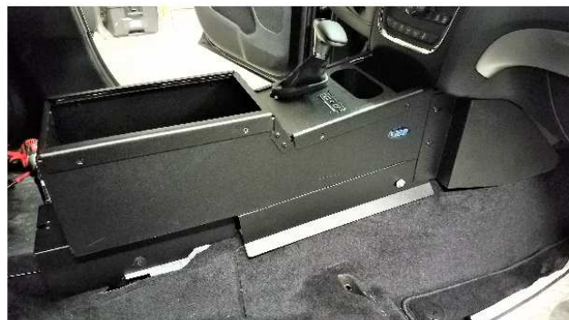
FIG 10 - CONSOLE AND SIDE PANELS INSTALLED
