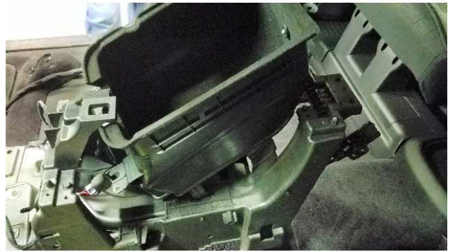
FIG 6 - POCKET TIPPED UP TO REMOVE E-BRAKE RELEASE MODULE
