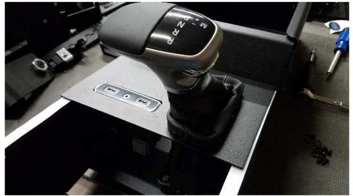
FIG 9 - SHIFTER HANDLE/BOOT AND USB MODULE INSTALLED INTO FACEPLATE
