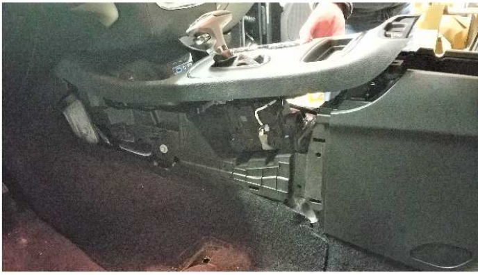
FIG 1 - Center Section Lifted, Side Panels Removed
