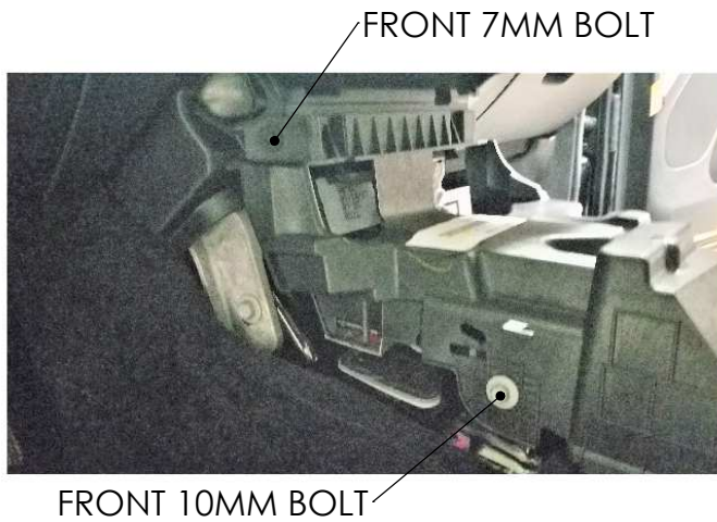
FIG 5 - FRONT CONSOLE STRUCTURE BOLTS
