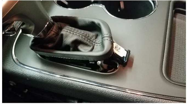
FIG 2 - Shifter Boot Unplugged and Trim Piece Removed
