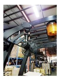
fan shown mounted on forklift overhead auard
