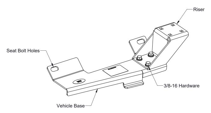
These instructions cover the installation of the 7160-1324 Gamber-Johnson vehicle base in 2019 and newer Ram 1500 to 3500 model trucks. This vehicle base is not compatible with older body style 2019 model year 'Classic' trim level trucks.
