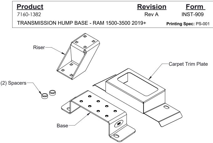
These instructions detail the installation of the Gamber-Johnson base, 7160-1382, into 2019 and newer Ram 1500-3500 trucks equipped with a center seat.
