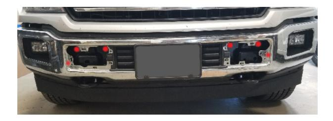
2. Remove tow hooks on both sides from vehicle (if necessary) by removing all (4) bolts with a 5/8"socket. Save all bolts and both nut plates for later use. (Extra bolts and nut plates have been provided in hardware bag for vehicles without tow hooks).
