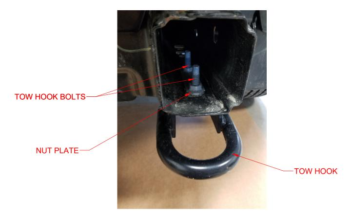
3. Install inner mounting brackets. Use factory bolt brackets and push nuts provided in hardware bag to hold upper bracket in place. Use factory (or provided) nut bracket and bolts to loosely attach lower bracket and tow hook, with bracket being between tow hook and vehicle frame. (If using factory bolts use 5/8" socket, if using provided bolts use 9/16" socket.) Repeat for both driver and passenger side.
