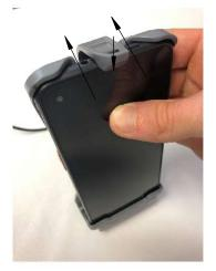
1.) Press up on the release button until the latch clears the top of the phone.
