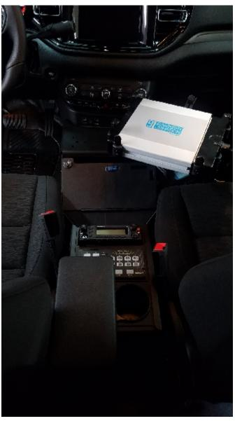
Note- Both versions of the console can be easily converted from printer mount to equipment mounting or vice versa without changing the entire console.
