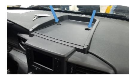
2. Place the GJ top tray inside the OEM tray and reinstall with the OEM bolts.
