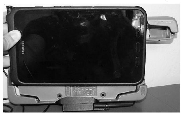
3. ROTATE AND LOWER THE TABLET INTO THE CRADLE PUSH BACK UNTIL IT SEATS
