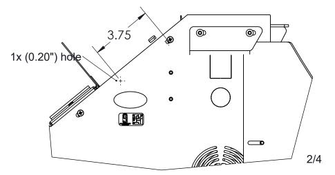
4. To install printer mount, align the 4 holes on the driver side and the 3 holes on the passenger side mount with the provide #10-32 hardware
