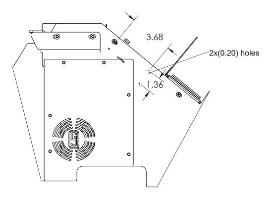
3. On The passenger side mark and drill as shown.
