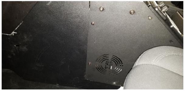
5. With the wings in place, the console can be attached to the vehicle with the OEM hardware (Figure 5). Torque bolt to OEM specs.
