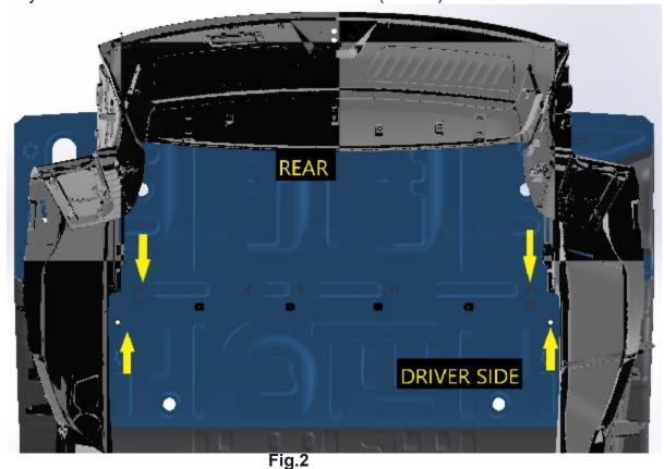
Shows the Top view of frame, Highlighted 4 arrows are mounting points for rear bracket/kicker rods
