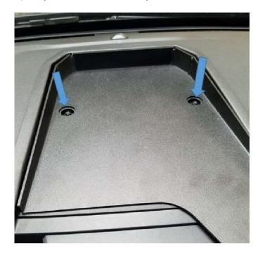
3. With the GJ Top Plate installed, install the middle vertical section of the On-Dash mount with provided 3/8" hardware.
