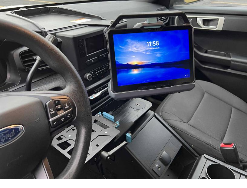
On the ease of access and increased control efficiency side, perhaps no other piece of equipment is as important as the center equipment console in a patrol vehicle. It is there to provide immediate, easy and efficient access to the officer for all of the essential controls that aren't inherently built into the vehicle. All communications and emergency notification functions are housed in that console.
