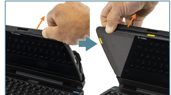
On both sides, push up on Top Latch Ridge & pull forward on back corner of Tablet
