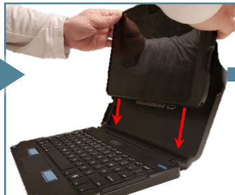
Insert Tablet into tray with Pogo Pins.
