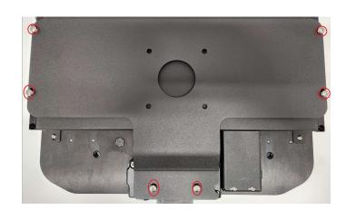
The standard mounting bracket that comes with the vehicle dock features an industry standard VESA 75mm bolt pattern. It must first be removed from the dock by unscrewing the 6x #10-24 screws attaching it to the dock. This allows easy mounting to many preexisting mounts as well as dedicated mounts from Gamber-Johnson.
