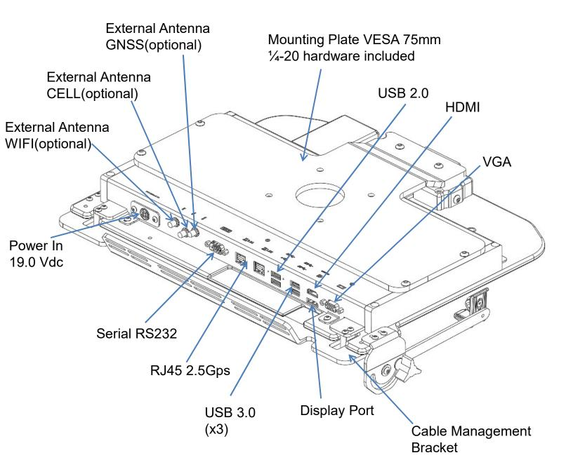
\*VGA port can only work alone, once HDMI or DP port plug in, VGA will not be functional
