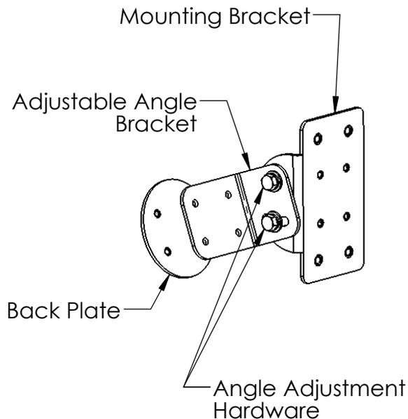
1. The mount is attached by drilling (4) 1/4" dia. holes in a flat surface where the mount will be attached. Use the adjustable angle bracket to mark the (4) locations before drilling. Verify nothing is behind the flat surface that can be damaged when you drill the holes. The hole pattern is 30mm x 38mm.
