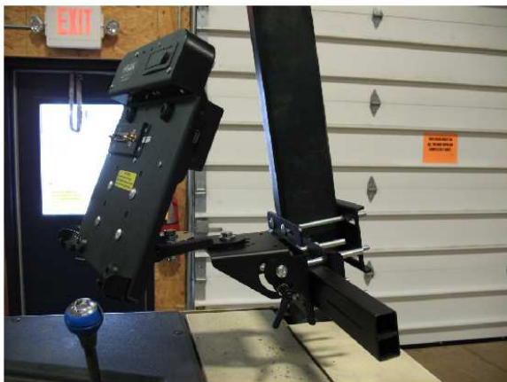
Views of pillar mount 7160-0364 mounted on an Extension tube to position the computer equipment in front of the fork truck
