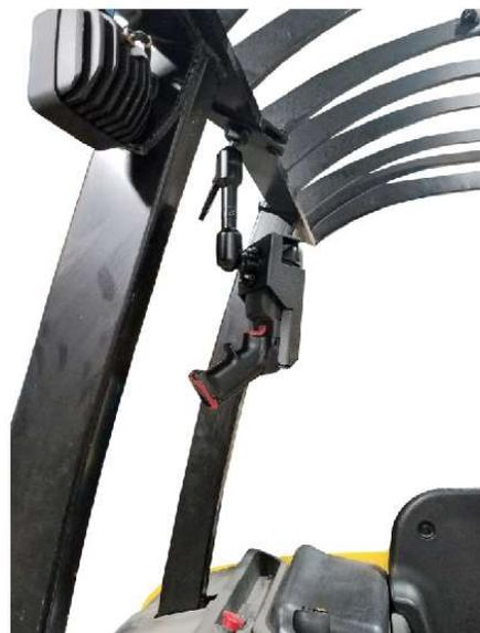
different view showing mount hanging from the overhead guard vs the previous photos mounted off the overhead guard leg
