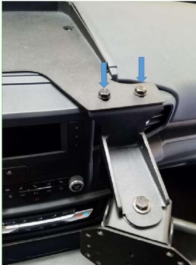
4. Remove the existing two bolts from the top plate of the GJ Low-Profile Console, then use the provided 1/4-20 allen head hardware to attach the leg of the On-Dash to the console as shown. Then, attach the upper part of the leg to the vertical section of the On-Dash mount.
