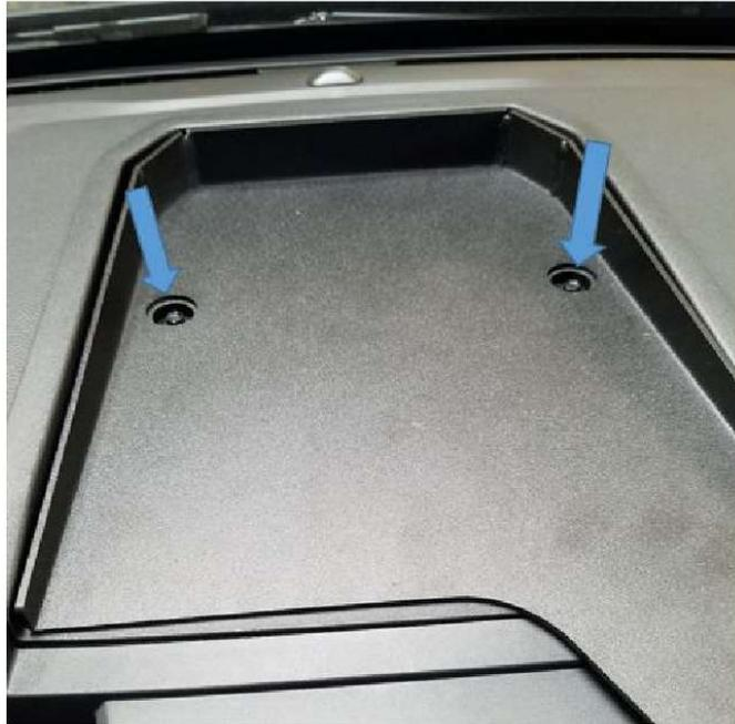
3. With the GJ Top Plate installed, install the middle vertical section of the On-Dash mount with provided 3/8" hardware.
