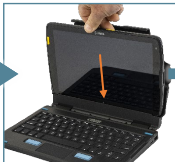
Insert Tablet into tray with Pogo Pins
