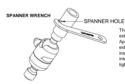
The spanner wrench is used to tighten extension tubes onto the joiner bodies. Apply epoxy thread locker EA 9460 on external and internal M20 threads, then insert the hook end of the spanner wrench into the hole of the extension tube to tighten the joint.
