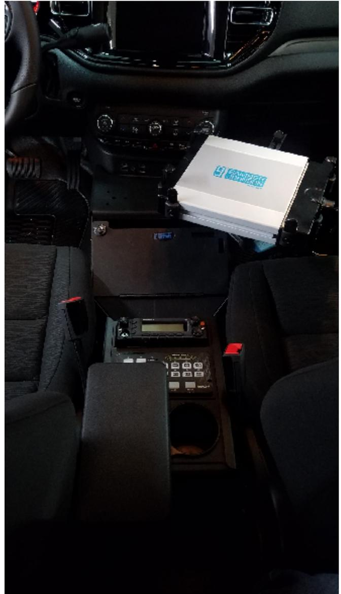
Note- Both versions of the console can be easily converted from printer mount to equipment mounting or vice versa without changing the entire console.
