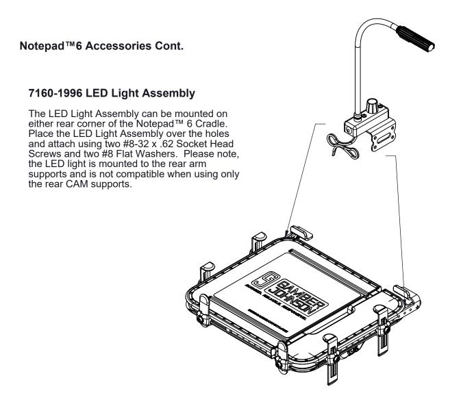
The LED is powered using the red and brown wires on the light base. The LED Assembly is designed to operate on 12 VDC.
