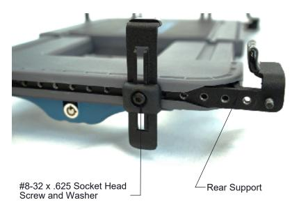
For additional support, insert the rear L-brace before inserting the rear supports and then attach with a #8-32 x .375 Socket Head Screw once the rear support is in the desired location
